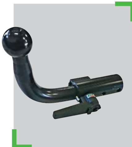
MODEL C Manually detachable ball with safety lock
